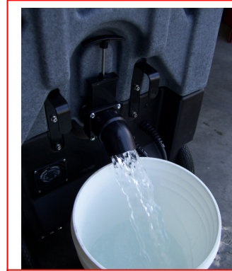
Drain Recovery Tank
