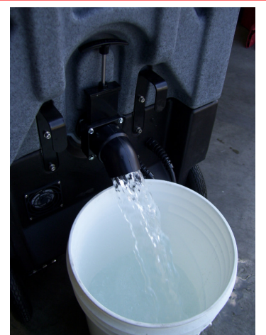
Draining the Recovery Tank
